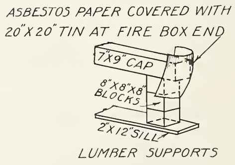
Figure 48. --Details of small hot-air kiln.
